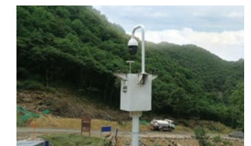
Venue construction PM 2.5 monitoring instruments on site
